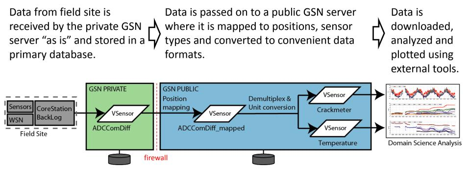
• All data from sensor nodes to backend is transmitted in packets
